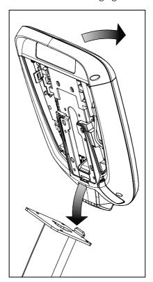
Figure 16: Console positioning on base unit
